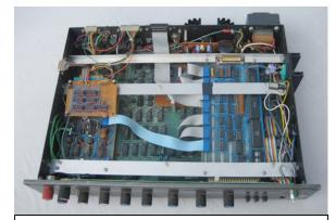
**Figure 8:** *Stargate* with Commodore removed, showing interface circuitry.
