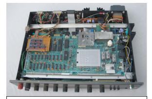
**Figure 7:** Ursa Major *Stargate* with additional circuitry, including Commodore 64 motherboard on top.
