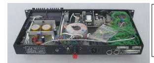
**Figure 11:** Trombone-propelled electronics rev. 2: open Bryston chassis (rear view) showing amplifier channel on left, SensorLab circuit boards on right.
