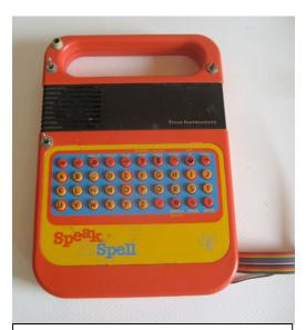
**Figure 6:** *Speak and Spell* modified to function as a computer speech synthesizer.
